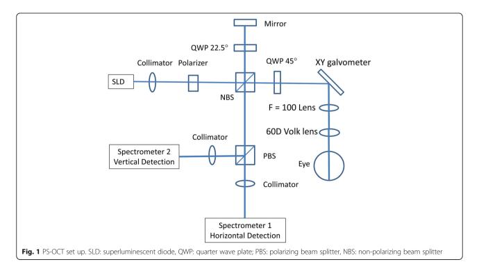
channels before reaching two identical spectrometers. The fringes of both vertical and horizontal reflected lights from the sample and reference mirror are detected and separated by these two spectrometers. Each of the spectrometers has a holographic diffraction grating (1200 lines/mm; Wasatch Photonics, Logan, UT) to span the fringe over 2048 sensor pixels on a line scan camera (Aviiva SM2 CL 2014, Atmel, San Jose, CA) with a projection lens (f = 180 mm).
