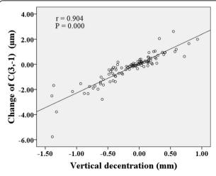
**Fig. 8** The correlation between vertical decentration and Zernike coefficient  $C_3^{-1}$  in (PCCP – OCCP)
