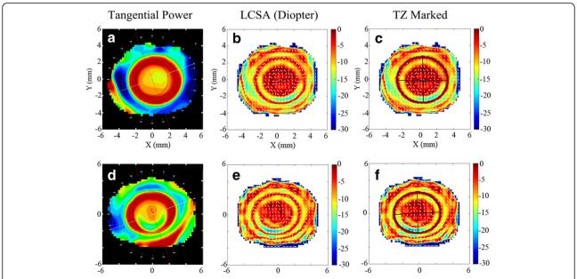
Fig. 1 Comparison between tangential power and LCSA for two subjects. a Tangential power, b LCSA and c LCSA with TZ marked of subject-I; d Tangential power, e LCSA and f LCSA with TZ marked of subject-II
